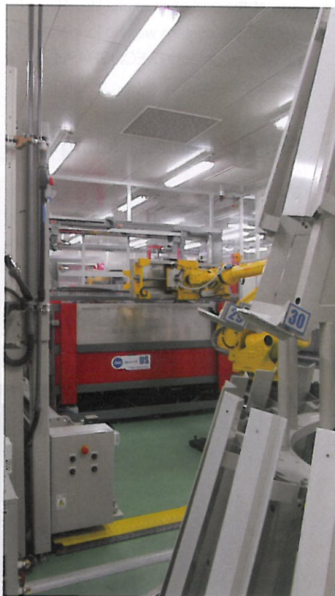
The Robot Arm Is Placing a Cylinder in the Ultrasound Cleaning Unit. The DAISAN Line Has Two Such Units
