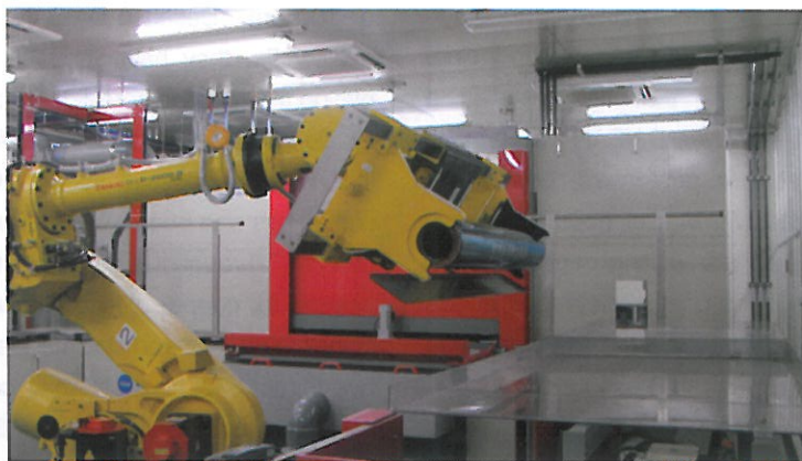
The Robot Arm Is Setting a Cylinder in the Etching Tank
